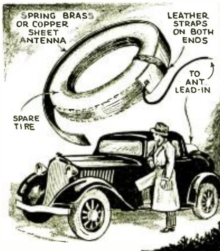
Two excellent suggestions for a car aerial for radio reception. One concerns the spare tire in the rear; the other is for side spares. On most cars these substitutes are as good as any.
